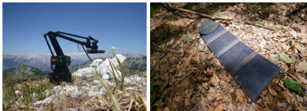
Figure 9 Portable robotic arm (uArm Swift Pro) with modular attachments for 3D printing, manipulation, laser cutting on a Slovenian mountain top. (right) Solar panel.
