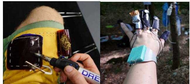
Figure 6 (left) heat-proof work surface built into one’s pants with magnets, sponges, and heat-proof Kapton film turn your lap into a workspace. (right) Perner-Wilson’s breadboard watches keep components at hand, and permit direct, wearable prototyping.
