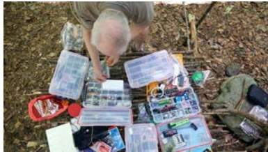
Figure 8 Hand-made lab bench from sticks containing water-tight, modular storage boxes filled with electronics and sensors.
